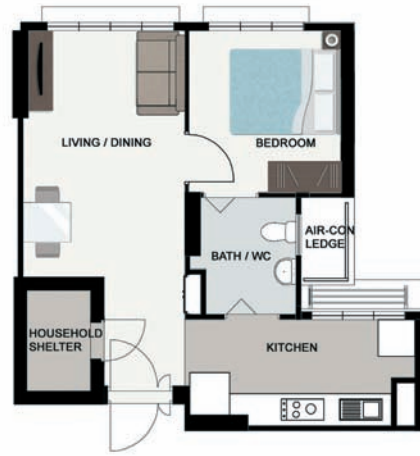
LAYOUT IDEAS FOR 2 ROOM (TYPE 2) APPROX. FLOOR AREA 47 sqm (Inclusive of internal floor area of 45 sqm and Air-con ledge)
