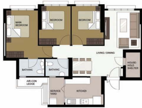
LAYOUT IDEAS FOR 4-ROOM APPROX. FLOOR AREA 93 sqm (inclusive of Internal Floor Area 90 sqm and Air-Con Ledge)
