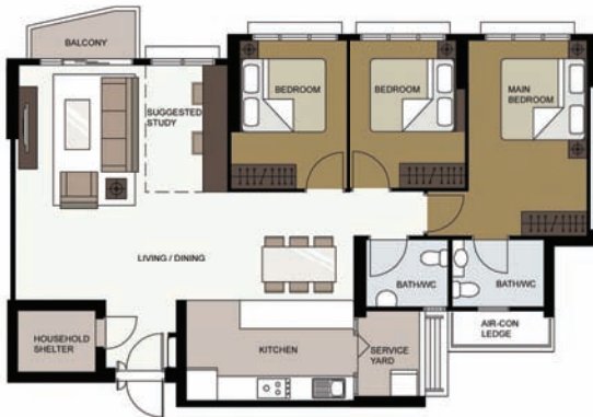
LAYOUT IDEAS FOR 5-ROOM APPROX. FLOOR AREA 116 sqm (inclusive of Internal Floor Area 113 sqm and Air-Con Ledge)
