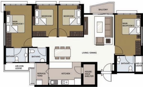
LAYOUT IDEAS FOR 3GEN FLAT APPROX. FLOOR AREA 123 sqm (inclusive of Internal Floor Area 118 sqm and Air-Con Ledge)
