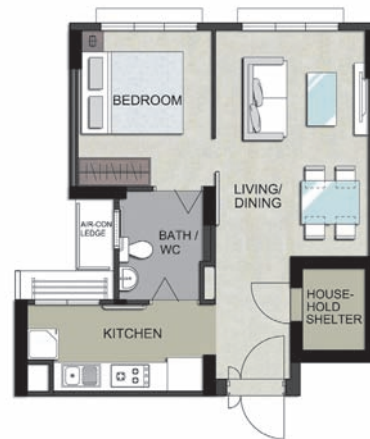
LAYOUT IDEAS FOR STUDIO APARTMENT (TYPE B) APPROX. FLOOR AREA 47 sqm (Inclusive of Internal Floor Area 45 sqm and Air-con Ledge)
