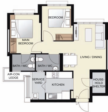
LAYOUT IDEAS FOR 3 ROOM APPROX. FLOOR AREA 68sqm (Inclusive of Internal Floor Area 65sqm and Air-Con Ledge)
