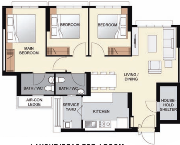
LAYOUT IDEAS FOR 4 ROOM APPROX. FLOOR AREA 92sqm (Inclusive of Internal Floor Area 90sqm and Air-Con Ledge)
