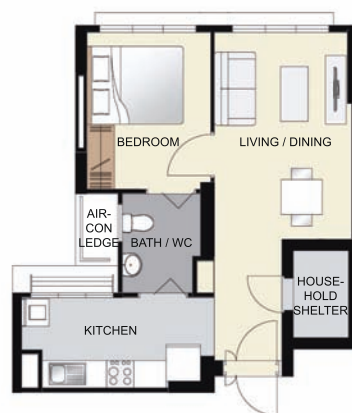
LAYOUT IDEAS FOR 2 ROOM (TYPE 2) APPROX. FLOOR AREA 47sqm (Inclusive of Internal Floor Area 45sqm and Air-Con Ledge)
