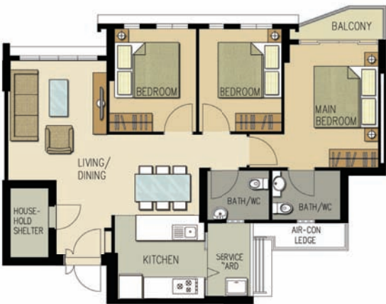
LAYOUT IDEAS FOR 4-ROOM APPROX. FLOOR AREA 93 sqm ( Inclusive of Internal Floor Area of 90 sqm and Air-Con Ledge )
