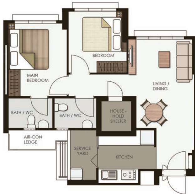
TYPICAL 3-ROOM FLOOR PLAN APPROX. FLOOR AREA 68 sqm (Inclusive of Internal Floor Area of 65 sqm and Air-Con Ledge)
