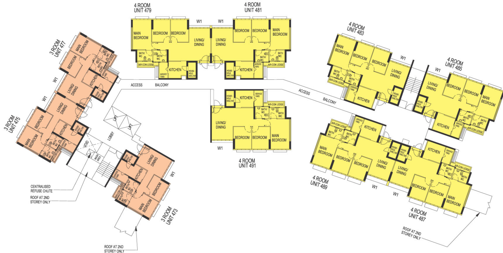
BLOCK 104A (2ND TO 15TH STOREY FLOOR PLAN)
