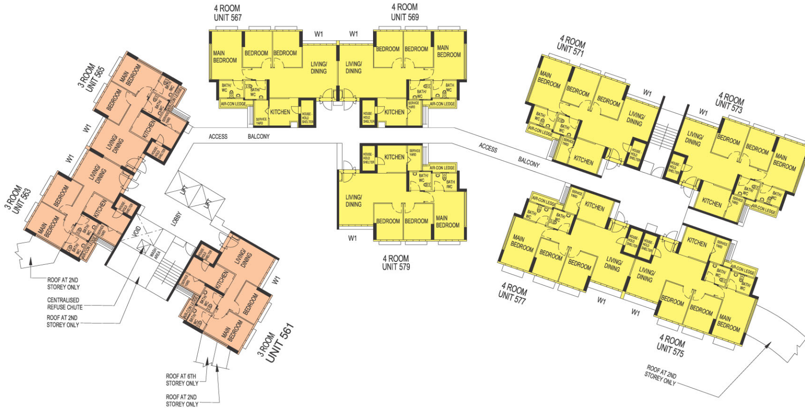
BLOCK 107A (2ND TO 4TH, 6TH TO 15TH STOREY FLOOR PLAN)
